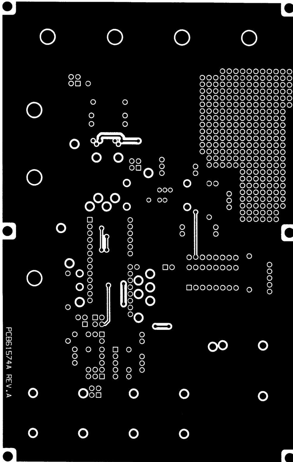
Figure 3. Top Ground Plane Layer (NOT TO SCALE)
