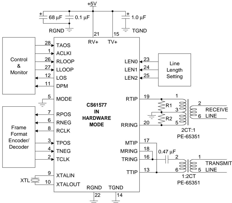
**Figure A2. 120 Ω, E1 Hardware Mode Configuration**
