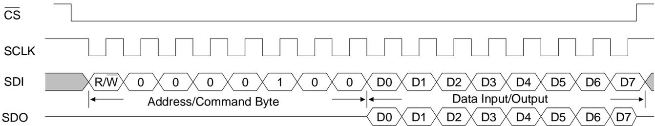
**Figure 13. Input/Output Timing**
