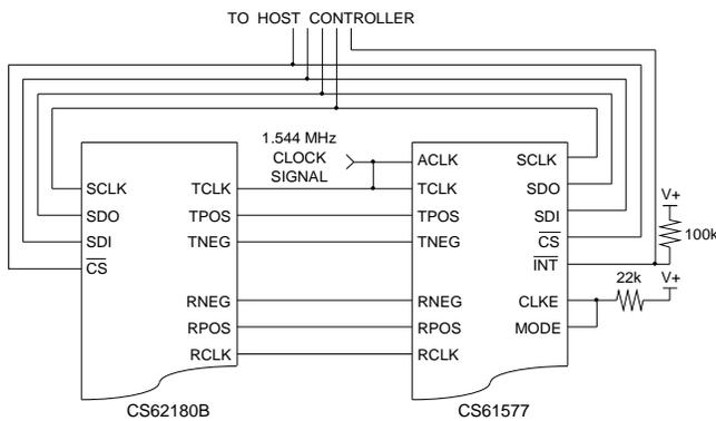
**Figure A4. Interfacing the CS61577 with a CS62180B
