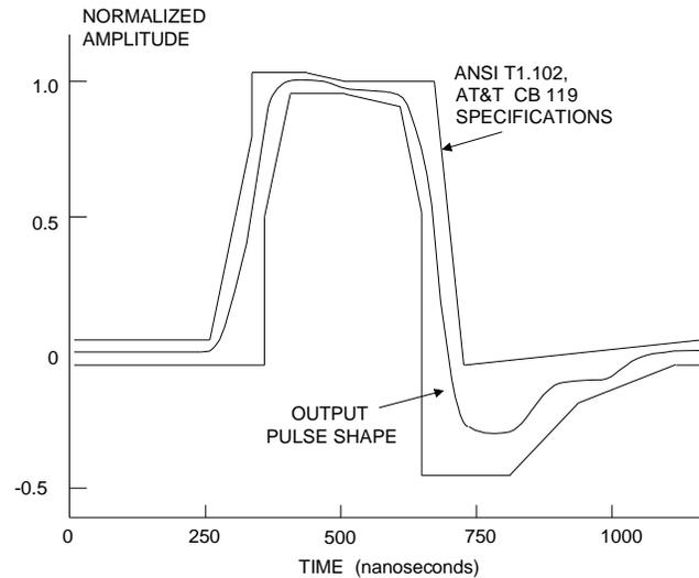
**Figure 8. Typical Pulse Shape at DSX-1 Cross Connect**
