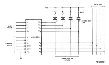
Convenient Register Content Monitor or Test Point
