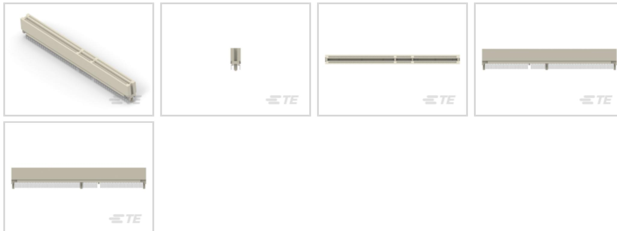
Connector System: **Board-to-Board**Number of Positions: **184**Centerline (Pitch): **1.27 mm [.05 in]**Termination Post & Tail Length: **3.56 mm [.14 in]**Contact Mating Area Plating Material Thickness: **[ 30  $\mu$ in ]**
