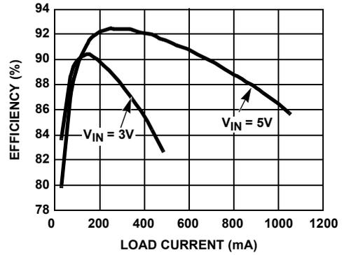
FIGURE 2. BOOST EFFICIENCY AT  $V_{OUT} = 12\text{V}$  (P-MODE)
