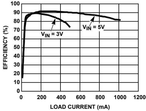
FIGURE 1. BOOST EFFICIENCY AT  $V_{OUT} = 12\text{V}$  (PI-MODE)
