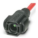
Device connector front mounting, Range of articles: SUNCLIX, housing material: PPE, color: black, number of positions: 1, min. conductor cross section: 6 mm², Connection method: Crimp, Contact connection type: Pin, cable length: 500
