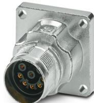
M17, Device connector front mounting, series: M17 PRO, straight, shielded: yes, for standard and ONECLICK fast locking system, No. of pos.: 8, contact connection type: Socket, Crimp connection, flange dimensions: 28 mm x 28 mm, coding: N, Item is lead-free in accordance with RoHS II without Exemption 6c (Pb < 0.1 %)
