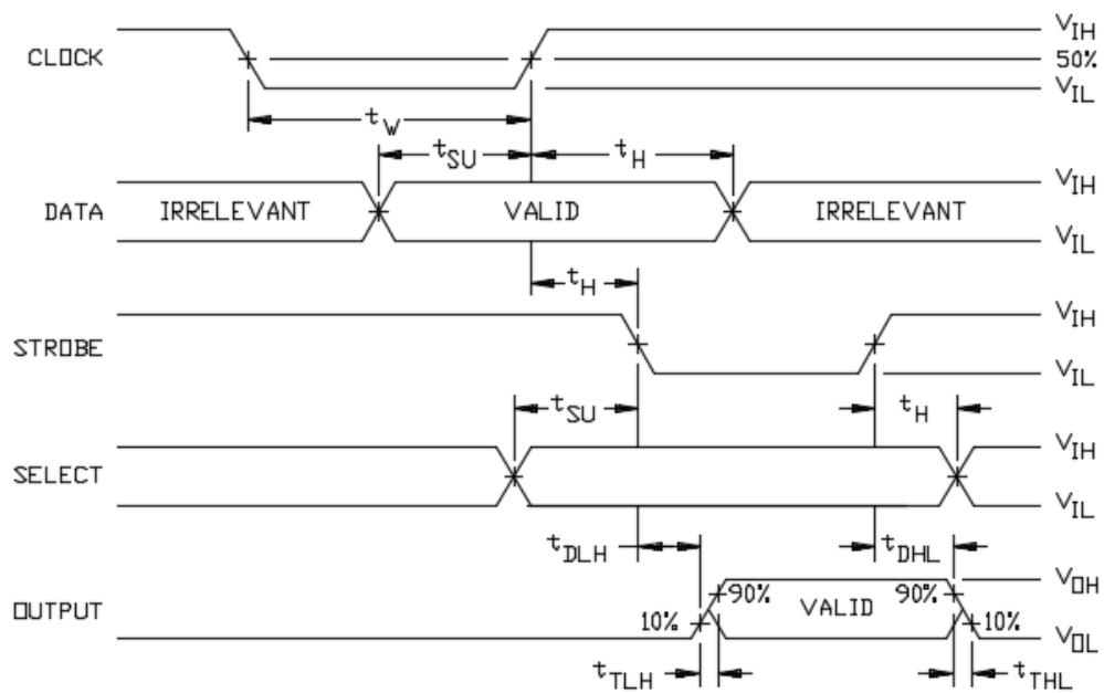
FIGURE 4. Switching waveforms.
