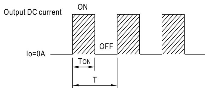
$$\text{Duty cycle}(\%) = \frac{T_{ON}}{T} \times 100\%$$
