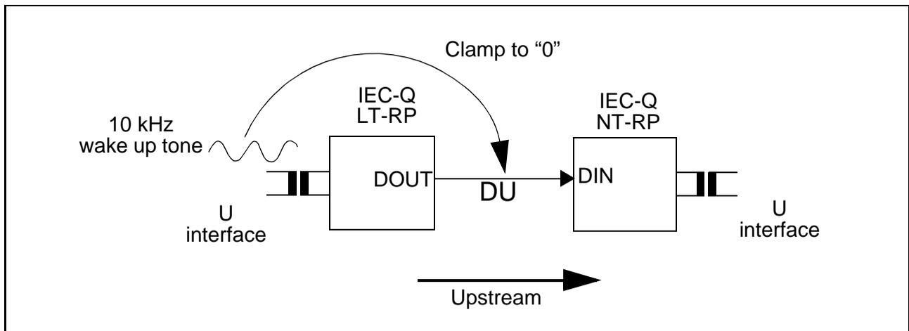
**Figure 6 Wake Up Indication in Repeater Power Down**
