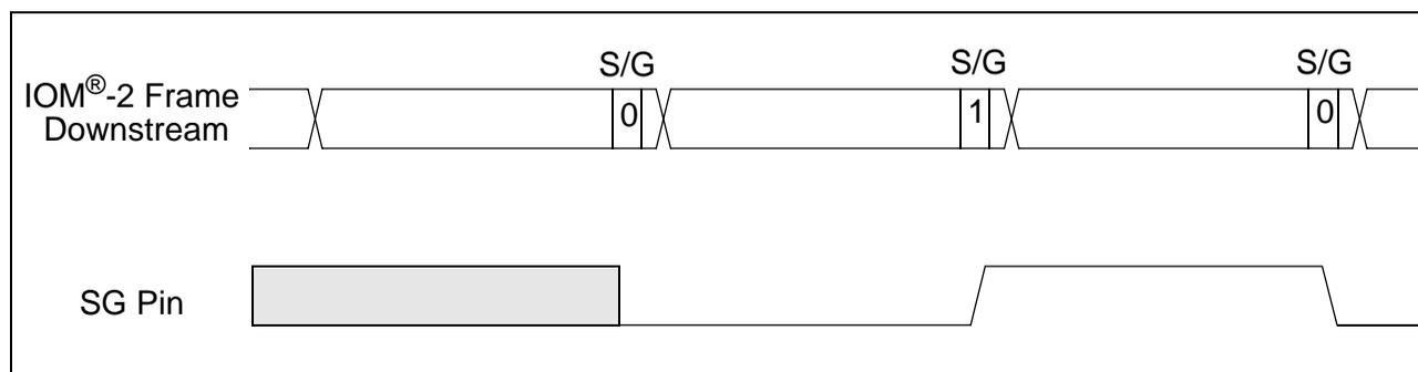
**Figure 12 S/G Bit Status on Pin S/G**
