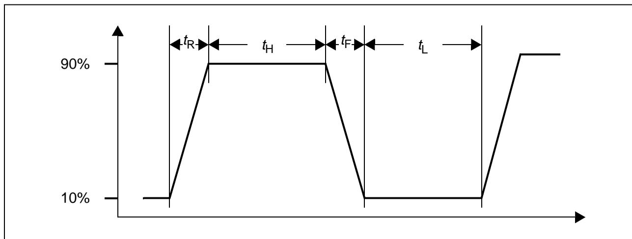
Figure 22 Dynamic Characteristics of CLS in NT-RP Mode
