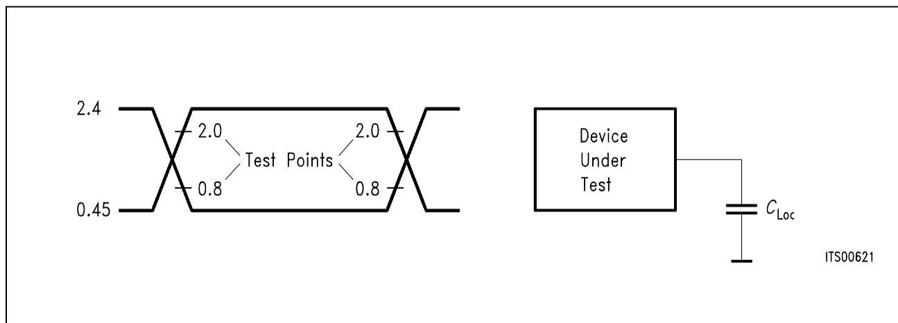
**Figure 13 Input/Output Wave Form for AC Tests**
