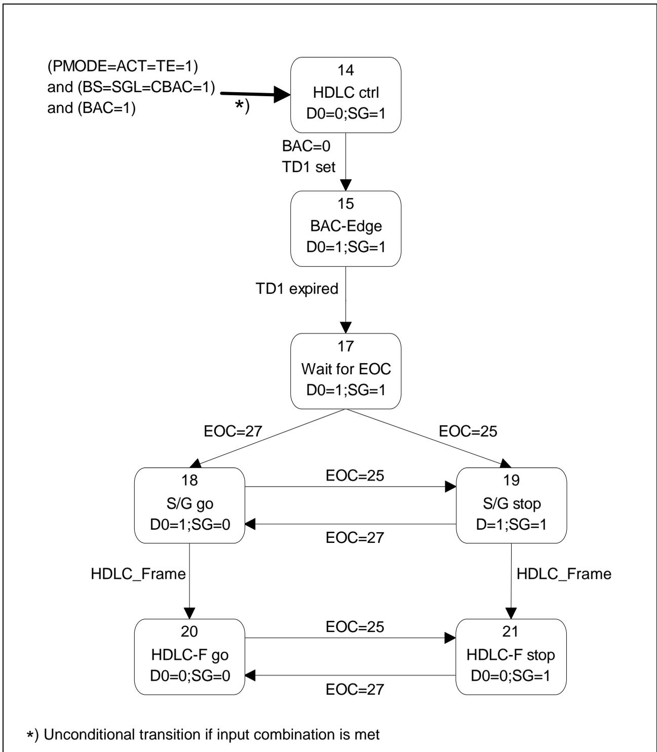
Figure 11 State Machine for S/G Bit Control (Part 3)
