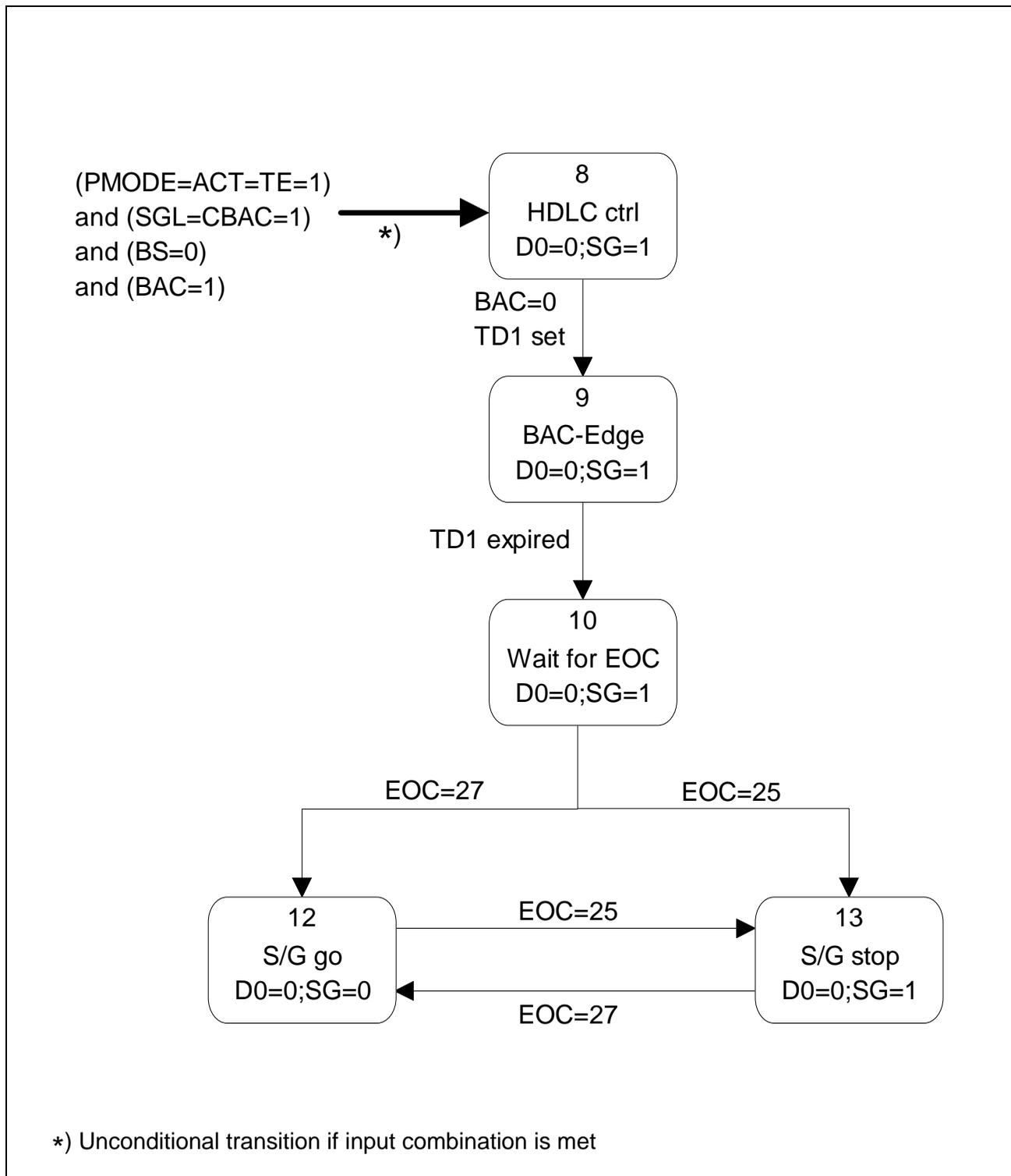
Figure 10 State Machine for S/G Bit Control (part 2)
