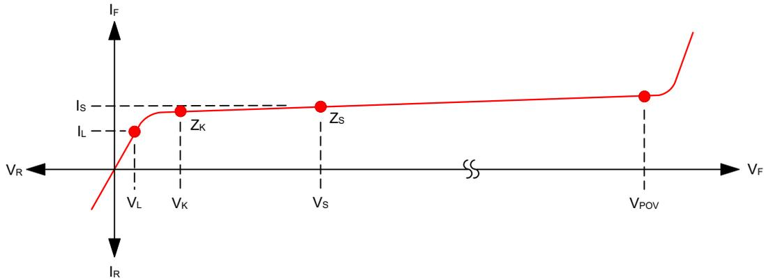
FIGURE 10. Current to voltage characteristics for CRD devices.
