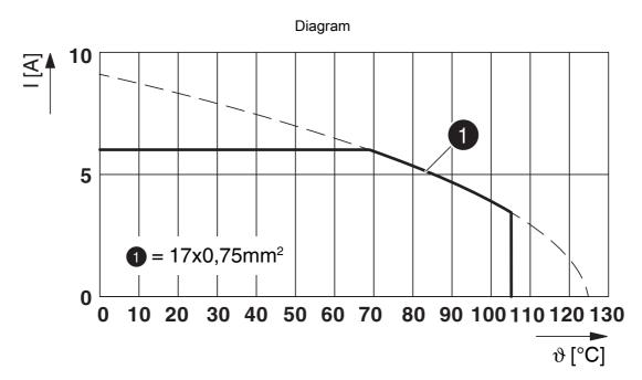
I = current strength,  $\vartheta$  = ambient temperature, 17x 6 A
