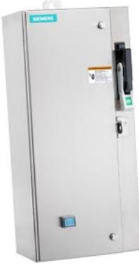
Non-reversing motor starter, Size 0, Three phase full voltage, Solid-state overload relay, OLR amp range 3-12A, Combination type, 30A fusible disconnect, 30A/250V fuse clip, Encl NEMA type 4X 304 S-Steel, Water/dust tight noncorrosive, Standard width enclosure
