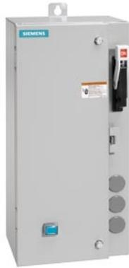
Non-reversing motor starter, Size 1, Three phase full voltage, Solid-state overload relay, OLR amp range 0.75-3.4A, Combination type, 3A circuit breaker, Enclosure NEMA type 4/12, Water/dust tight for outdoors, Standard width enclosure
