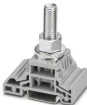
High-current connector, nom. voltage: 1000 V, nominal current: 269 A, number of connections: 1, connection method: Bolt connection, Rated cross section: 120 mm<sup>2</sup>, mounting type: NS 35/7,5, NS 35/15, color: gray
