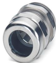
Cable gland, material for screw connection: Brass, nickel-plated, application: EMC, external cable diameter 9 mm ... 13 mm, shielding: yes, connecting thread: M20 x 1.5, color: silver, with O-ring
