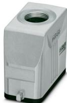
Sleeve housing D15, for single locking latch, material: Die-cast aluminum, salt water resistant, cable outlets: 1, straight, 1x M20, height: 56 mm, cable gland: none, Standard
