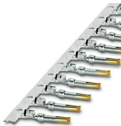
Crimp contact, Socket, rolled, Taped product, number of pieces per reel: 10000, contact diameter: 1 mm, crimp range: 0.22 mm<sup>2</sup> ... 0.56 mm<sup>2</sup>, Item is lead-free in accordance with RoHS II without Exemption 6c (Pb < 0.1 %)
