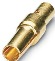
Crimp contact, Socket, turned, Single contact, contact diameter: 1 mm, crimp range: 0.14 mm<sup>2</sup> ... 0.56 mm<sup>2</sup>, Contact release tool not necessary for the 12- and 17-pos. crimp versions of the M23-PRO series, Alternative product in accordance with RoHS II without Exemption 6c (Pb < 0.1 %) item no.: 1241093
