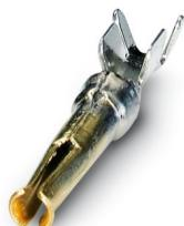
Crimp contact, Socket, rolled, Single contact, contact diameter: 1 mm, crimp range: 0.22 mm<sup>2</sup> ... 0.56 mm<sup>2</sup>, Single contact, Item is lead-free in accordance with RoHS II without Exemption 6c (Pb < 0.1 %)
