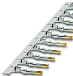
Crimp contact, Socket, rolled, Taped product, number of pieces per reel: 500, contact diameter: 1 mm, crimp range: 0.22 mm<sup>2</sup> ... 0.56 mm<sup>2</sup>, Item is lead-free in accordance with RoHS II without Exemption 6c (Pb < 0.1 %)
