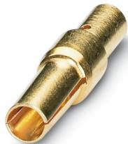
Crimp contact, Socket, turned, Single contact, contact diameter: 1 mm, crimp range: 0.08 mm<sup>2</sup> ... 0.22 mm<sup>2</sup>, Contact release tool not necessary for the 12- and 17-pos. crimp versions of the M23-PRO series, Alternative product in accordance with RoHS II without Exemption 6c (Pb < 0.1 %) item no.: 1241093
