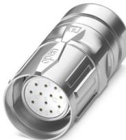
M23, Cable connector, series: CA, straight, shielded: yes, SPEEDCON, No. of pos.: 16, Direction of rotation: Standard, contact connection type: Socket, Crimp connection, cable diameter range: 6 mm ... 10 mm, coding: N, Alternative product in accordance with RoHS II without Exemption 6c (Pb < 0.1 %) item no.: 1243626
