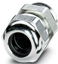
Cable gland, material for screw connection: Brass, nickel-plated, external cable diameter 7 mm .. . 10.5 mm, shielding: no, connecting thread: Pg11, series: RC
