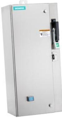
Non-reversing motor starter, Size 0, Three phase full voltage, Solid-state overload relay, OLR amp range 0.25-1A, 110V 50Hz / 120V 60Hz coil, Combination type, 30A fusible disconnect, 30A/250V fuse clip, Encl NEMA type 4X 304 S-Steel, Water/dust tight noncorrosive, Standard width enclosure
