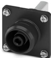
Connector, Range of articles: BPC, housing material: PA, color: black, number of positions: 1, min. conductor cross section: 95 mm<sup>2</sup>, max. conductor cross section: 120 mm<sup>2</sup>, rated voltage: 1500, rated current: 350 A, Connection method: Screw/Solder connection, Contact connection type: Pin
