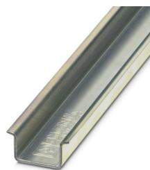
DIN rail, unperforated, Pack of 25 (50 m), similar to EN 60715, material: Steel, galvanized, passivated with a thick layer, Standard profile, color: silver
