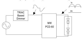
Under direct driving, the power supply will work in "constant current mode (CC)" and output voltage of the power supply will be clamped by sum of forward voltage (VF) of the LED strip.
