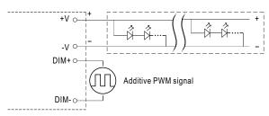
"DO NOT connect "DIM- to -V"
