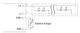
"DO NOT connect "DIM- to -V"
