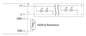
"DO NOT connect "DIM- to -V"
