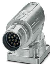
M17, Device connector front mounting, series: M17 PRO, angled rotatable, shielded: yes, for standard and ONECLICK fast locking system, No. of pos.: 17, contact connection type: Socket, Crimp connection, flange dimensions: 28 mm x 28 mm, coding: N, Item is lead-free in accordance with RoHS II without Exemption 6c (Pb < 0.1 %)
