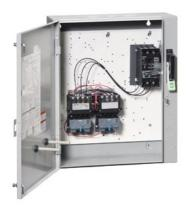
2-speed 3-phase motor starter Size 0 Two separate windings Constant horsepower Solid-state overload relays Low SPD OLR range 3-12A High SPD OLR range 5.5-22A 110V 50HZ / 120V 60HZ coil Combination type 25Amp circuit breaker Enclosure NEMA type 4/12 Water/dust tight for outdoors
