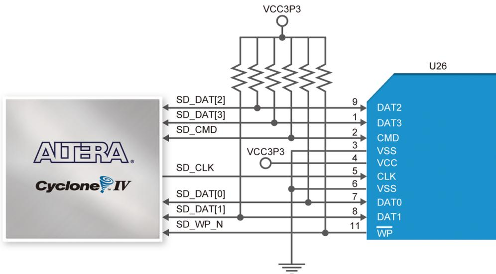
**Figure 4-37** Connections between FPGA and SD Card Socket
