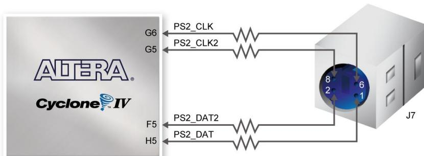
Figure 4-25 Connection between FPGA and PS/2
