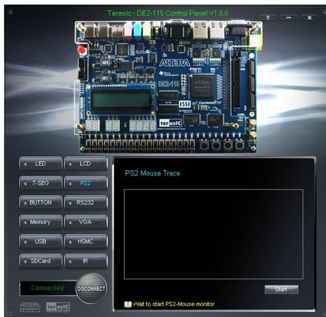
**Figure 3-9 PS/2 Mouse Monitoring Tool**
