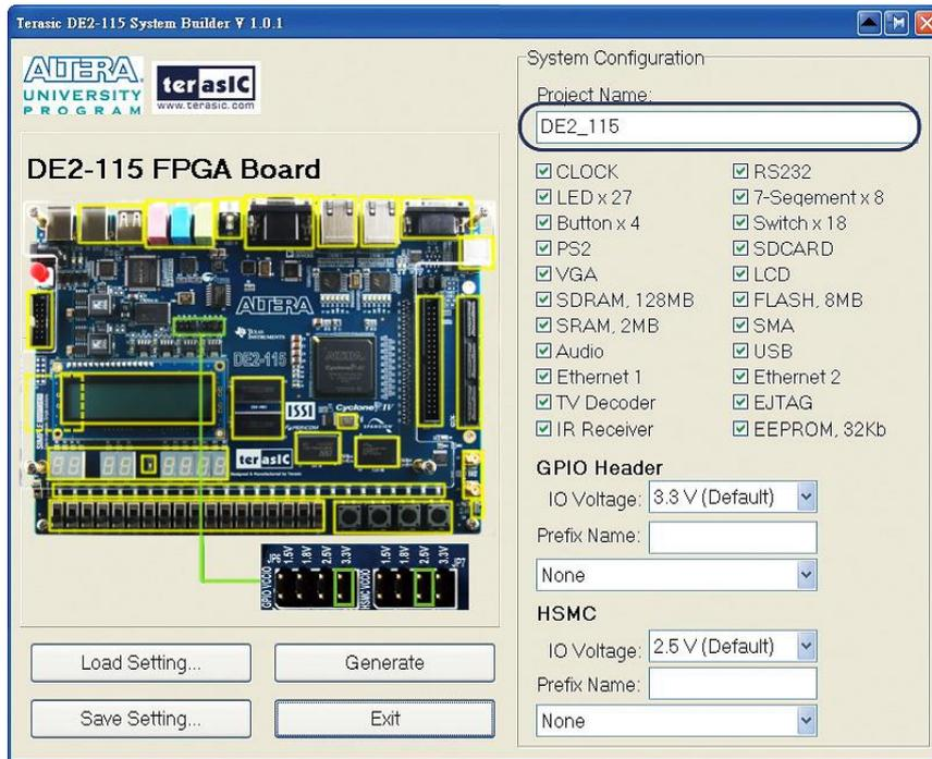
**Figure 5-3 The DE2-115 Board Type and Project Name**
