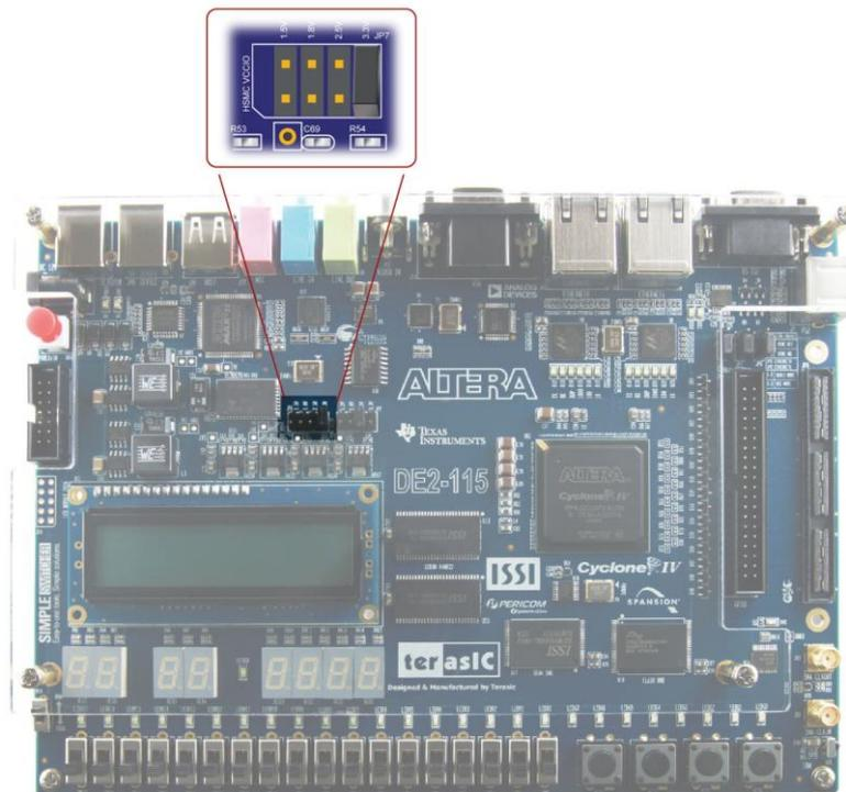
**Figure 4-17** GPIO VCCIO supply voltage setting header
