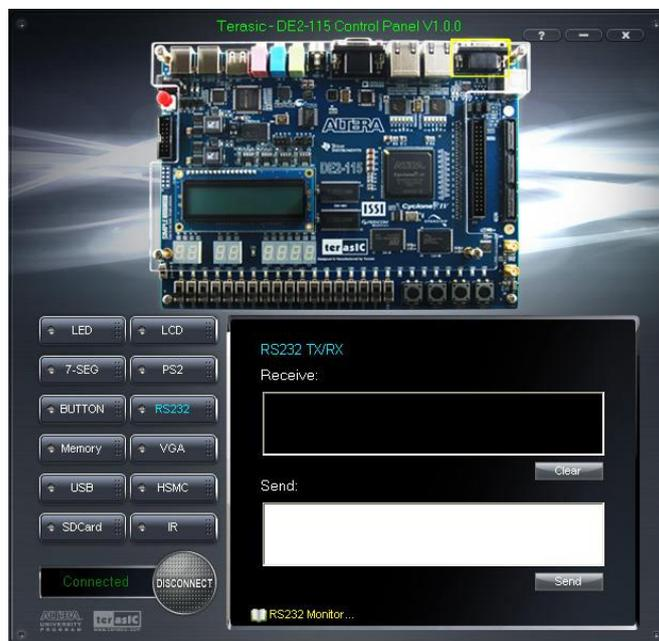
Figure 3-11 RS-232 Serial Communication
