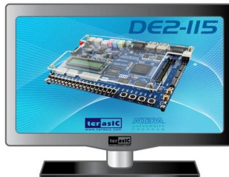
Figure 2-4 The default VGA output pattern
