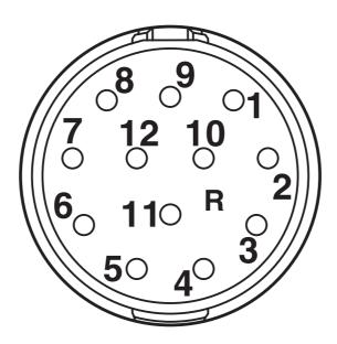
Contact chamber numbering (view of plug-in side), socket counter direction
