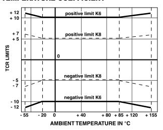
The temperature coefficient is guaranteed between -20  $^{\circ}$ C to +85  $^{\circ}$ C.
