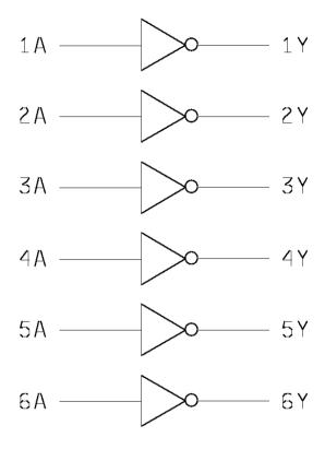
FIGURE 3. Logic diagram.
