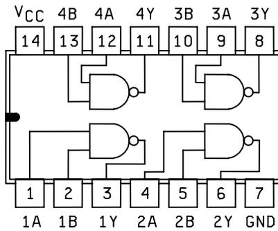
FIGURE 1. Terminal connections and logic diagrams - Continued.
