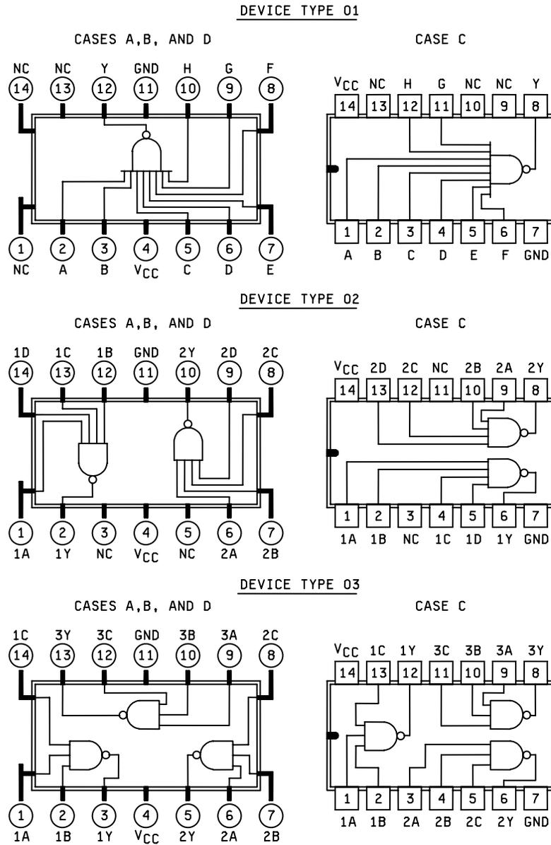
FIGURE 1. Terminal connections and logic diagrams.
