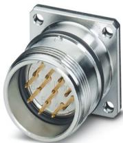
M23, Device connector front mounting, series: RC, straight, shielded: yes, Screw locking mechanism, No. of pos.: 12, Direction of rotation: Standard, contact connection type: Pin, Solder cup, Flat gasket, 4x Ø 2.7 mm, flange dimensions: 25 mm x 25 mm, Panel thickness min.: 1 mm, coding: N, Alternative product in accordance with RoHS II without Exemption 6c (Pb < 0.1 %) item no.: 1240752
