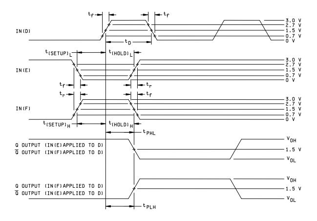
FIGURE 5. Synchronous waveforms and test circuit for device type 01 - Continued.
