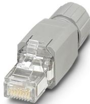
RJ45 connector, design: RJ45, degree of protection: IP20, number of positions: 6, CAT5, material: Plastic, connection method: Insulation displacement connection, connection cross section: AWG 26- 23, cable outlet: straight, VARAN
