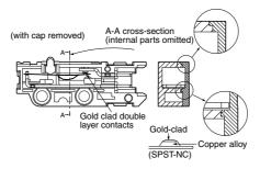
The contact arrangement is available in two types, the SPST-NC and the SPST-NO. • The lever position is available in two types.
