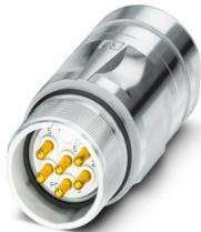
M23, Coupler connector, series: CA, straight, shielded: yes, for standard and SPEEDCON interlock, No. of pos.: 8+1, Direction of rotation: Standard, contact connection type: Pin, Crimp connection, cable diameter range: 3 mm ... 14.5 mm, coding: N, Alternative product in accordance with RoHS II without Exemption 6c (Pb < 0.1 %) item no.: 1244050
