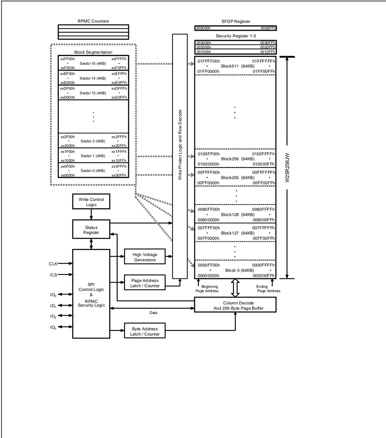
Figure 2. W25R256JW Serial Flash Memory Block Diagram
