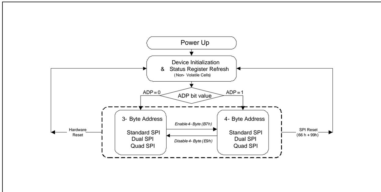
Figure 3. W25R256JW Serial Flash Memory Operation Diagram
