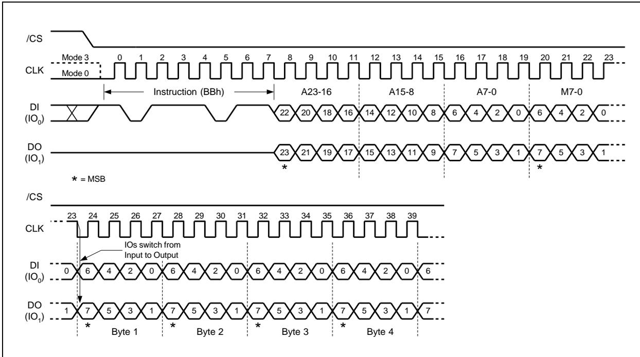
Figure 22a. Fast Read Dual I/O Instruction (Initial instruction or previous M5-4 ≠ 10)
