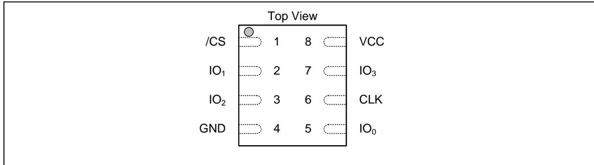
Figure 1a. W25R256JW Pad Assignments, 6X5 & 8x6-mm (Package Code P & E)
