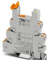
14 mm PLC basic terminal block for high continuous currents with Push-in connection, without relay or solid-state relay, for mounting on DIN rail NS 35/7,5, 1 changeover contact, input voltage 12 V DC
