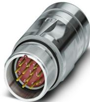
M23, Coupler connector, series: CA, straight, shielded: yes, for standard and SPEEDCON interlock, No. of pos.: 17, Direction of rotation: Standard, contact connection type: Pin, Crimp connection, cable diameter range: 4 mm ... 6 mm, coding: N, Alternative product in accordance with RoHS II without Exemption 6c (Pb < 0.1 %) item no.: 1243945
