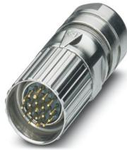
M23, Cable connector, series: CA, straight, shielded: yes, Screw locking mechanism, No. of pos.: 16+2+FE, Direction of rotation: Standard, contact connection type: Pin, Crimp connection, cable diameter range: 3 mm ... 14.5 mm, coding: N, Alternative product in accordance with RoHS II without Exemption 6c (Pb < 0.1 %) item no.: 1245007
