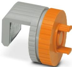
The optional holding device ensures the Rogowski coil is securely seated on busbars with a thickness of 10 ... 15 mm. During installation, the coil housing is pushed onto the flange of the holding device and snaps in automatically.
