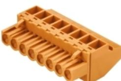
Female plugs with clamping-yoke connection for connecting wires with a right-angle (90° or 270°) outlet direction. The female connectors provide space for labelling and can be coded. Fastened by means of a flange or release latch. They also provide an integrated plus/minus screw, protection against faulty insertion of the wire, and they are delivered with open clamping yokes. HC = High Current.
