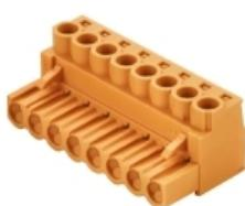
Female plug with clamping-yoke screw system for connecting wires with straight (180°) outlet direction. The female connectors provide space for labelling and can be coded. Fastened by means of a flange or release latch. They also provide an integrated plus/minus screw, protection against faulty insertion of the wire, and they are delivered with open clamping yokes. HC = High Current.
