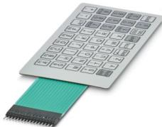
Membrane keypad, self-adhesive, silver conduction technology, 45 keys, embossed, 4 colors, connecting cable: 77 mm, with crimp female connector, pitch: 2.54 mm, operating temperature: -20°C ... 70°C
