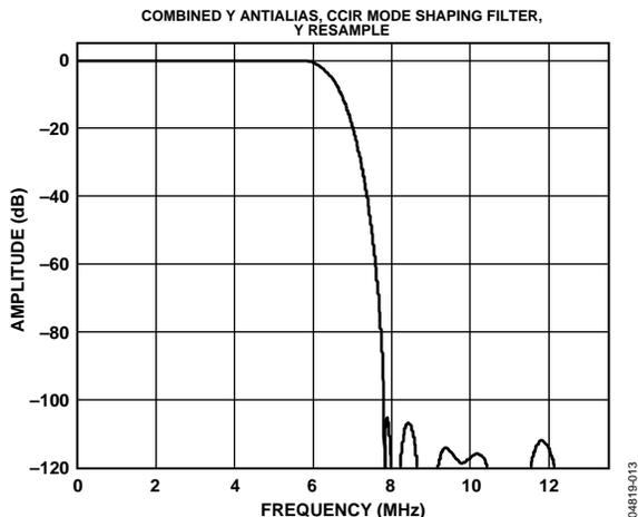
Figure 13. Y S-VHS 18 Extra Wideband Filter (CCIR 601 Compliant)
