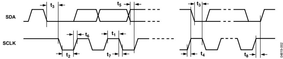
Figure 2. I<sup>2</sup>C Timing
