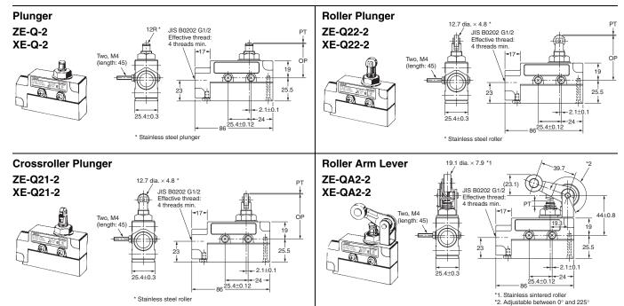
Note: 1. Unless otherwise specified, a tolerance of  $\pm 0.4$  mm applies to all dimensions.
