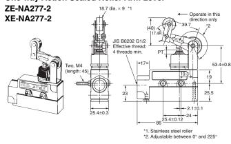
Note: 1. Unless otherwise specified, a tolerance of  $\pm 0.4$  mm applies to all dimensions.
