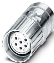
M23, Cable connector, series: CA, straight, shielded: yes, Screw locking mechanism, No. of pos.: 6, Direction of rotation: Standard, contact connection type: Socket, Crimp connection, cable diameter range: 6 mm ... 10 mm, coding: N, Alternative product in accordance with RoHS II without Exemption 6c (Pb < 0.1 %) item no.: 1243774
