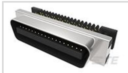
Connector Style: **Plug**Shielded: **No**Connector System: **Cable-to-Cable**Number of Positions: **80**Centerline (Pitch): **1.27 mm [.05 in]**
