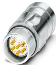
M23, Coupler connector, series: CA, straight, shielded: yes, for standard and SPEEDCON interlock, No. of pos.: 8+1, Direction of rotation: Standard, contact connection type: Pin, Crimp connection, cable diameter range: 6 mm ... 10 mm, coding: N, Alternative product in accordance with RoHS II without Exemption 6c (Pb < 0.1 %) item no.: 1243998
