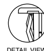
DETAIL VIEW VH1, VH3 & VH5 HOLE PLUGS (No wing serrations for ease of removal)
