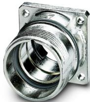
Panel mounting base, series: RC, straight, Screw locking mechanism, M23, Axial O-ring, 4x Ø 3.2, shielded: yes, Alternative product in accordance with RoHS II without Exemption 6c (Pb < 0.1 %) item no.: 1240308
