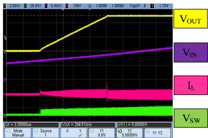
Figure 21. Start-Up Transition at No Load
