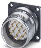
M23, Device connector rear mounting, series: RC, straight, Screw locking mechanism, Flat gasket, 4xM3, Panel thickness min.: 2.7 mm, Panel thickness max.: 3.5 mm
